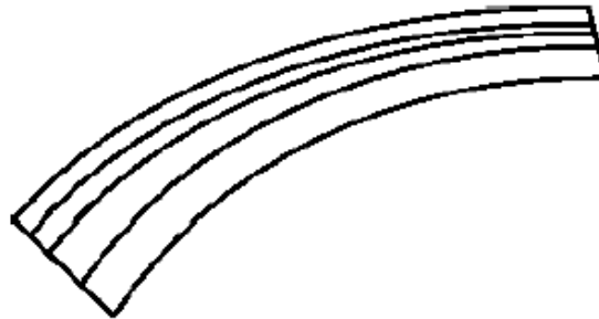
A two dimensional version of the streamtube
